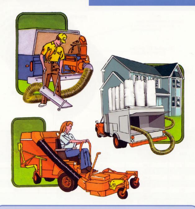
Kanaflex 630 ED standard and 660 YD heavy-duty duct hoses are specially designed for demanding blowing and ducting applications. They are perfect for cleaning ducts, for blowing cotton, straw, wood chips, grain dust or street refuse, and for leaf and grass collection.
